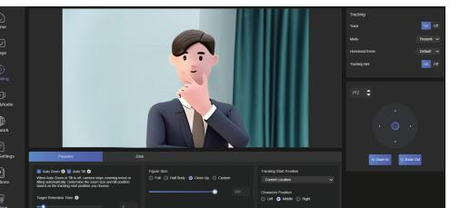
4) Custom: freely set the tracking target size. When the size value is high, the tracking target will be larger in close-up image, which may make the camera not keeping up when the tracking target moves quickly, as shown below:
